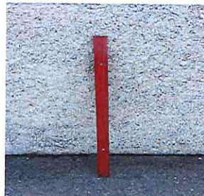
Straight Guard Rail Post Used on Superhigh Capacity Bunks Mounted on the inside of the Bunk
